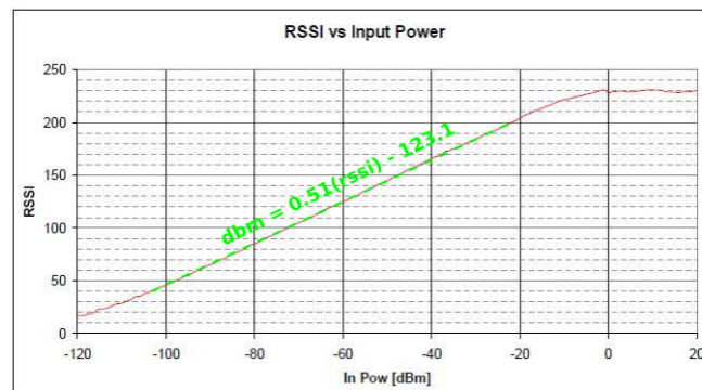
Figure 31. RSSI Value vs. Input Power
