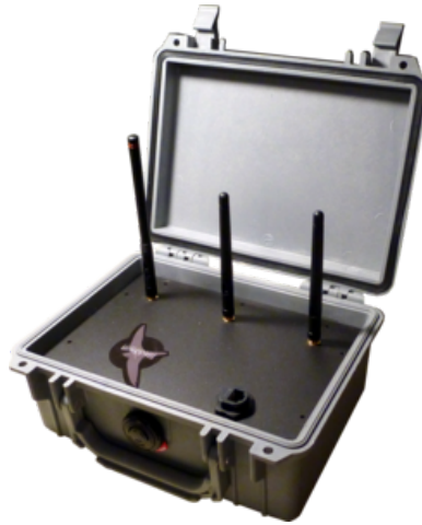
Figure 4.4: The RF emitting beacon.
